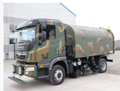
Truck Mounted Road Sweeper
