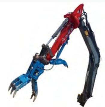
Excavator's 360° infinite rotary type boom(Arm)
